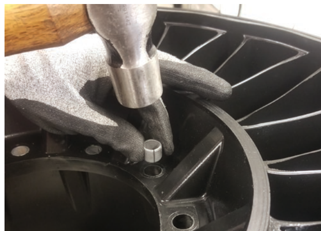
Above: Tapping in a compression limiter using a small hammer.
